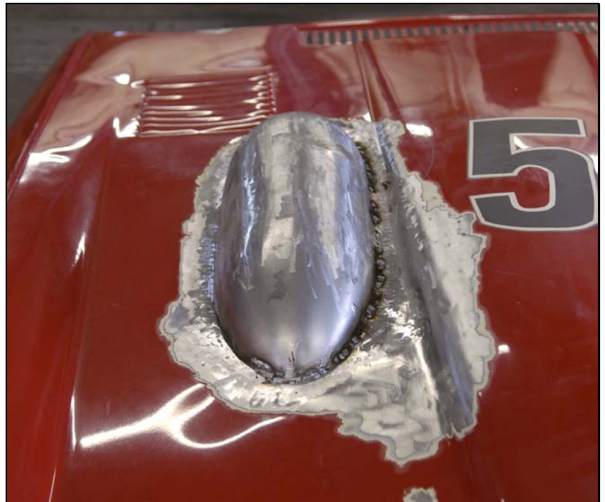
Blister is inserted and welded. Left side of picture shows welded areas carefully being ground away. Right side of picture is the before grinding view. Also notice the three sections of the blister are now gone. Further finishing and painting will make it look like an OEM design. See the first and last pictures in this article.
