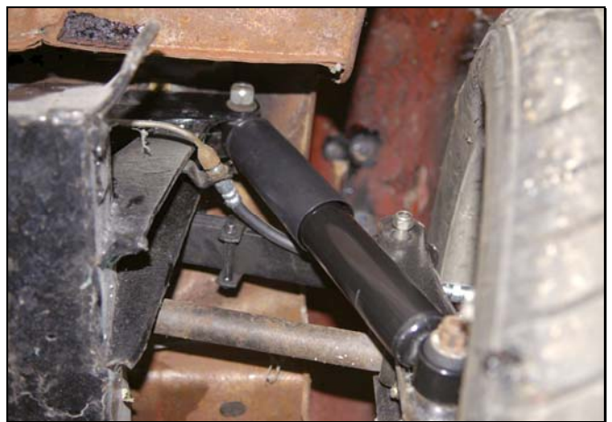
New rear shocks and transverse leaf spring shore up our car's ragged rear. Yes, that's a new brake hose.
