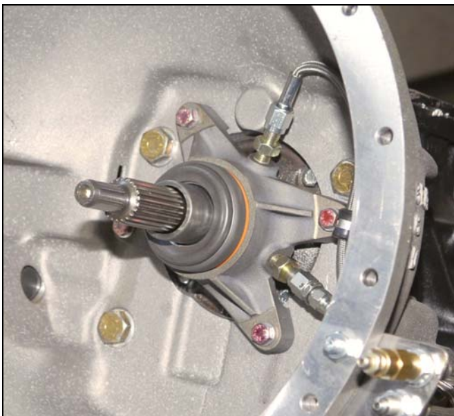
Close up of installed coaxial release bearing. Note: (in right lower corner) upper bleeder fitting and lower hydraulic connector.
