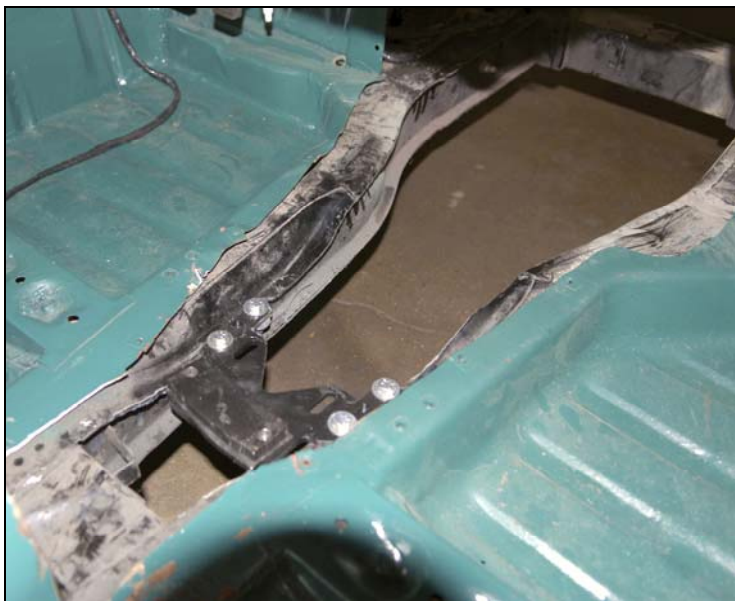
Sheet metal is removed from tunnel area and a new transmission rear mount is installed.
