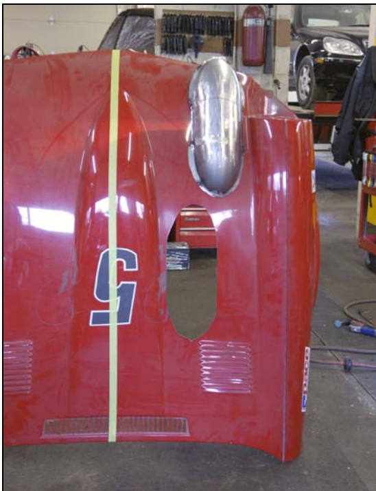
If you look closely at the fabricated blister at the top of the hood you can still see its three component sections. They will soon disappear with further finishing. The hole is cut awaiting blister insertion.
