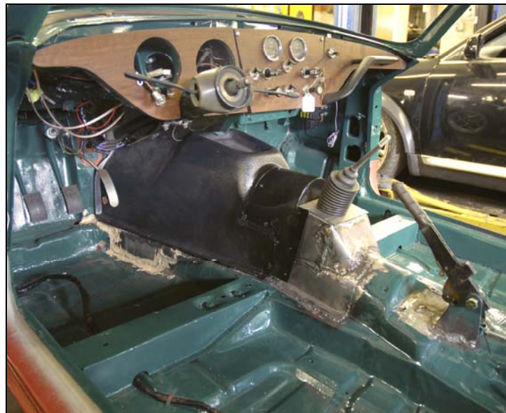
Modifying the tunnel to fit the gearshift takes many hours of careful fabrication and welding. Mods to the black plastic transmission cover require more time. Moving the handbrake lever back requires yet more cutting, grinding and welding, plus shortening of the cable. At times it seemed like it would never end, but the final product justified all the work.
