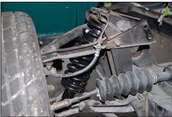
New front shocks, springs and a now dusty rebuilt rack and pinion help our worn track racer track well on the street. New brake hose is the sign of a well done brake job.
