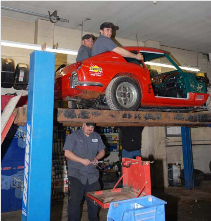
The car must be loaded to proper ride height before the new suspension components can be torqued. Yes, it was as silly as it looks. But effective!
